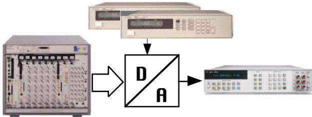
Used to extract linearity (differential an integral). The pattern generator send a digital ramp signal to DUT and synchronize measurement device.
