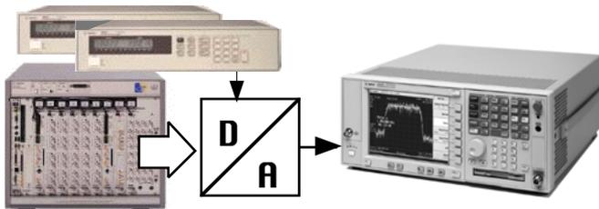
Using a Performance Spectrum Analyzer enables to get THD, SFDR and Noise results.
