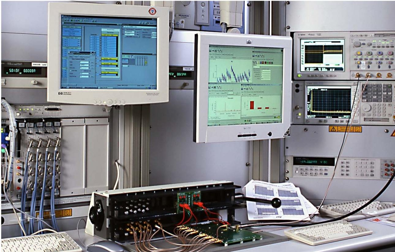
Today components used in wireless or video applications require specialized test equipment from bench, fine characterisation for 10 to 14 bits converters with hundreds of Megahertz sampling frequency is an heavy task for lab engineers.
